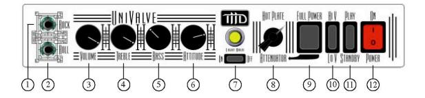
**1. MORE Input:** This jack fits a standard 1/4" mono shielded instrument cable. If you use a stereo cable, the sleeve signal will be ignored. Do not use speaker cable into this input. The MORE input is the high gain input, meaning that both preamp gain stages will be engaged in order to pass the hottest possible signal to the power section.
